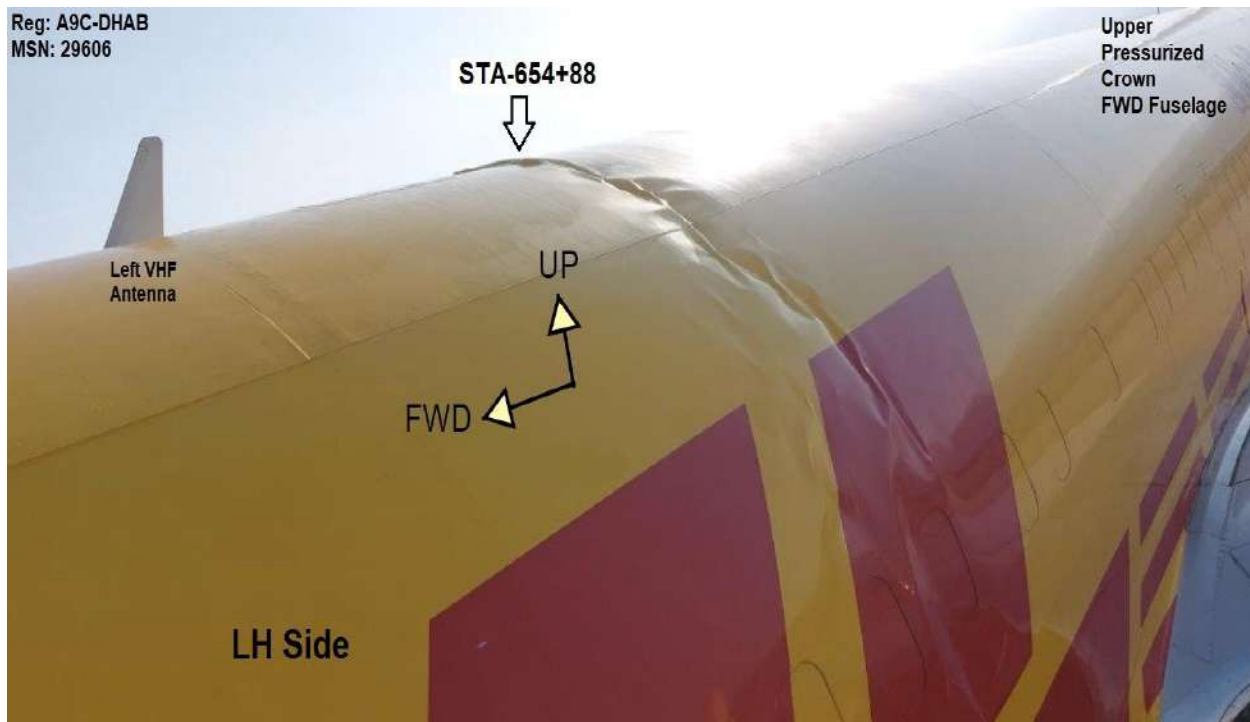
Figure 1: Top and LH side view of the damage to the fuselage
