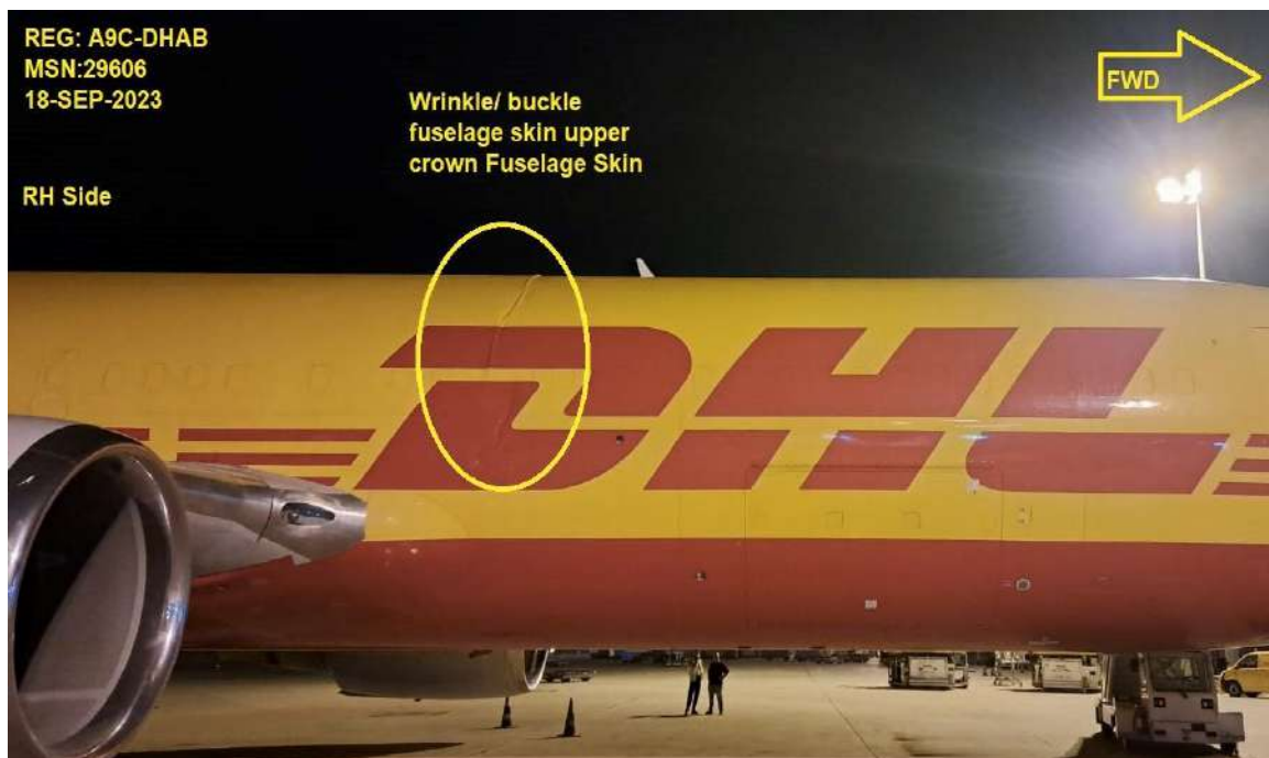
Figure 6: Wrinkle/buckled fuselage Skin upper crown fuselage damage
