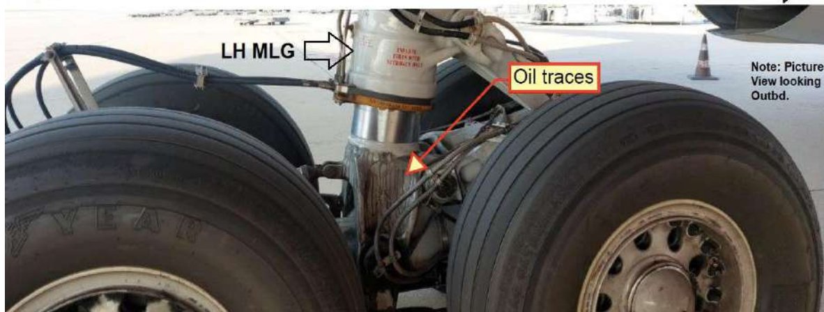
Figure 2: LH Main Landing Gear oil traces
